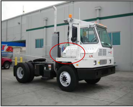
PINC Yard Hound: RFID Reader on Yard Truck
