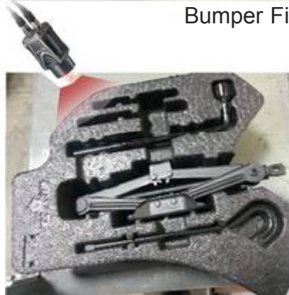
Vision detects unfilled slots in a Jack Kit
